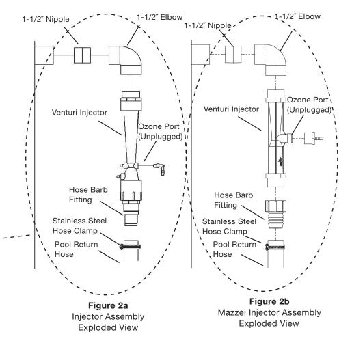
Figure 2 Installation Schematic for Injector Assembly
