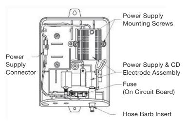
Figure 6 Internal component locations
