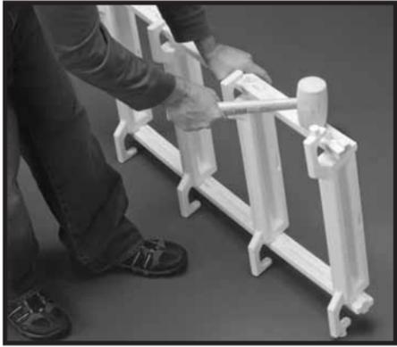
**#4:** Repeat step two to align the rectangular holes in the remaining tread connector with the tabs on the slide treads. Turn slide ladder assembly on edge and tap tread connector down until firmly seated.
