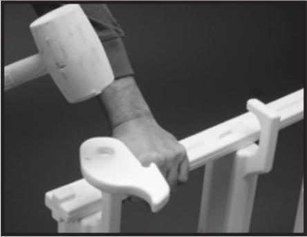
**#5:** Align the hole in the locking cam with the round tab on the locking slide tread and tap down. It may require several hits with rubber mallet. Repeat on the other side.
