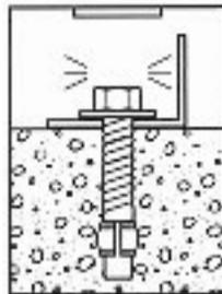
6. Expand anchor by tightening nut 3 to 5 turns. Once anchor is set remove nut and install a lock washer, item # (3), and retighten nut to a torque of 55 ft.-lbs.
