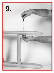
Using two 1/4-20 x 2" bolts and two acorn nuts fasten the extension boots to the ladder legs.
