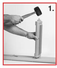
Push the end of one of the treads into one of the keyhole slots of the ladder leg. It may be necessary to tap the tread into the slot using a mallet or hammer
