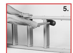
Attach one of the ladder legs to the opposite ends of the four treads making sure that the curved upper ends are both facing in the same direction. Tap the treads into place making sure that they are fully seated into the keyhole slots
