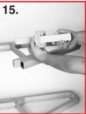
Lubricate the adjustable tubes with a small amount of dish detergent or silicone spray and slide the tube up through the mounting block as shown.
