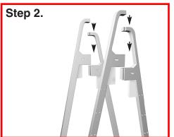
Slide the handrail/ legs together as shown. Apply liquid soap or spray lubricant to aid assembly.
