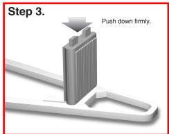
Place one handrail/leg assembly on a clean flat surface and push the deck platform protrusions in the opening.
