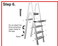
Slide five upper treads into position so they are resting on the double nubs of the legs (as shown in the diagram). Secure the treads to the legs using the #10 x 1-1/4" screws (two per tread), through the pre-drilled holes.
