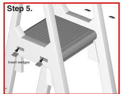
Insert the four wedges that were saved from step 1, into the top of the openings as shown.
