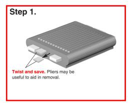
IMPORTANT: Remove the wedges from the deck platform protrusions and <u>SAVE</u> for step 5.
