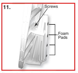
Place the Base and Brace into position, centered, on the bottom and fourth treads of the ladder. Install the four (4) #10 x 1-1/4" screws (included in hardware pack) on a slight angle, first in the Upper brace, then in the Lower Base. Install the self-adhering foam strips to the Large Barrier Section as shown in diagram.
