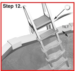
Place the ladder in the pool and fill legs with water through the openings with a hose. Then plug the holes using the four push in plugs. Tilt it so the air is released from all the submerged treads.
