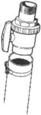
**6** Connect the pool suction plumbing between the skimmer, pool outlet and the pump.
