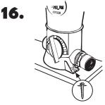
For best results use Phillips pan head screws through the mounting holes at the POOL FROG<sup>®</sup>Cycler base to secure the POOL FROG<sup>®</sup>Cycler into a treated wood base.
