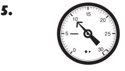
• Check the pool's filter gauge often and periodically clean filter per the manufacturer's directions. A dirty filter will slow the flow of water which could hamper proper circulation.
