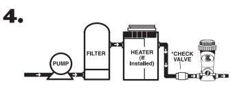
If using a POOL FROG<sup>®</sup> Bac Pac, isolating the POOL FROG<sup>®</sup> Cycler by installing a corrosion resistant check valve is recommended.
