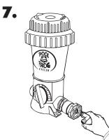
Screw elbow into reducer bushings on both sides.
