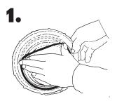
· Hold cap in front of you upside down with the o-ring groove facing up. Place one end of o-ring into cap groove at the point closest to you. Hold o-ring down with the thumb and forefinger of one hand.
