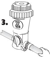
Insert PVC pipe into male adapters with a twisting action. Hold in place 5 to 10 seconds to bond.
