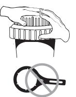
• Replace cap by hand only. **DO NOT OVER TIGHTEN.**
