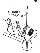
Use Phillips pan head screws through the mounting holes at the POOL FROG<sup>®</sup> Cycler base to secure the POOL FROG<sup>®</sup> Cycler into a treated wood base.
