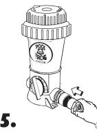
Insert reducer bushing into male adapter on both sides. Hold in place 5 to 10 seconds to bond.
