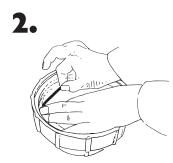
• Take hold of the far end of the o-ring with the thumb and index finger of the other hand. Roll o-ring slightly back towards you as you stretch the o-ring into the remainder of the cap groove.
