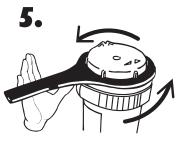
• Use the cap tool included with POOL FROG<sup>®</sup> Cycler to loosen cap by hitting the handle with the flat of your hand counter clockwise. If using the POOL FROG<sup>®</sup> Bac Pac, stand back to avoid inhaling chlorine fumes.
