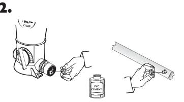
Following PVC cement directions brush PVC cement on the inside of the male adapters and to ends of the pipe .
