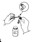
Following pipe thread sealant directions, brush sealant on to elbow threads.
