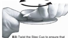
**B3)** Twist the Step Cup to ensure that the mushroom ring has entirely cleared the wall thickness. If it has, the suction cup should rotate freely.
