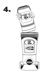
• Remove the POOL FROG® Mineral Reservoir and discard in trash. Even if you hear spent minerals inside, it is no longer effective. Replace with a new POOL FROG® Mineral Reservoir in the spring.
