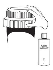
• Lubricate o-ring with the silicone lubricant that came with your POOL FROG® Mineral Hybrid. Do not use petroleum based lubricants. Replace the cap loosely.
